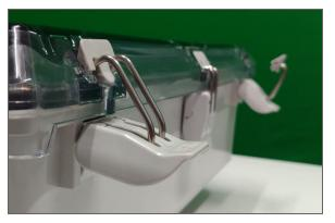
2. Lower the lever until flat against the surface of the enclosure as shown in the following image.
