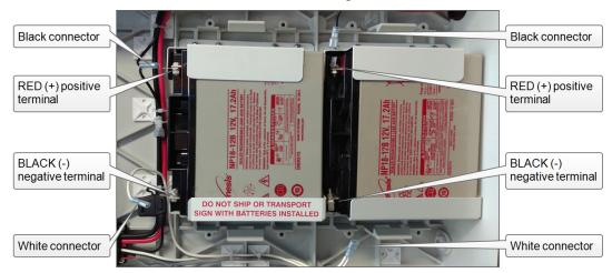
• Slide the white connector onto the BLACK (-) negative terminal.
