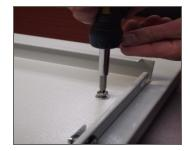
Figure 8: Attaching the sign bracket.
