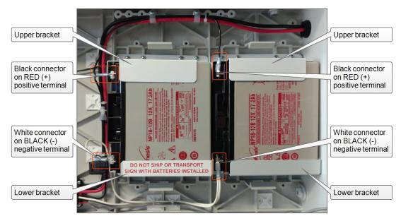
Figure 21: Lead acid battery inserted and connected
