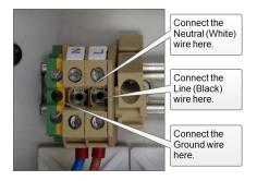
Figure 14: AC power supply terminal block
