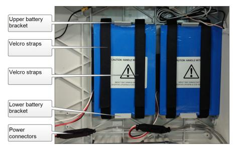
Figure 20: Lithium battery inserted and connected
