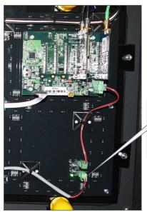
To reset the sign, disconnect this plug, wait a couple of seconds, then reconnect it.
